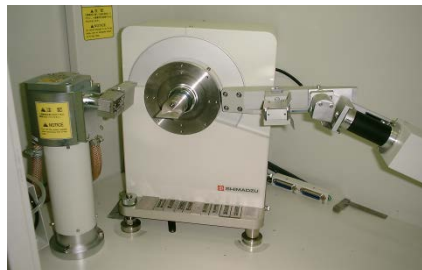
Fig. 3 The sample holder of XRD –Diffractometer [XRD 6000]
